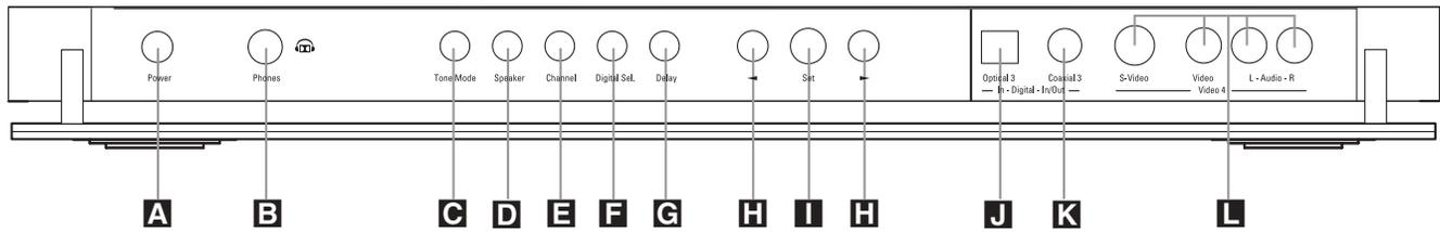
The following controls and jacks are located behind the front-panel door. To open the door, place the edge of a finger on the left or right edge of the panel and gently swing the door down towards you.
